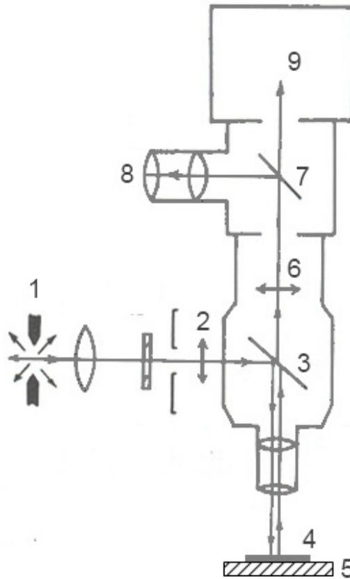
Fig.4. Scheme of the magneto-optic setup
