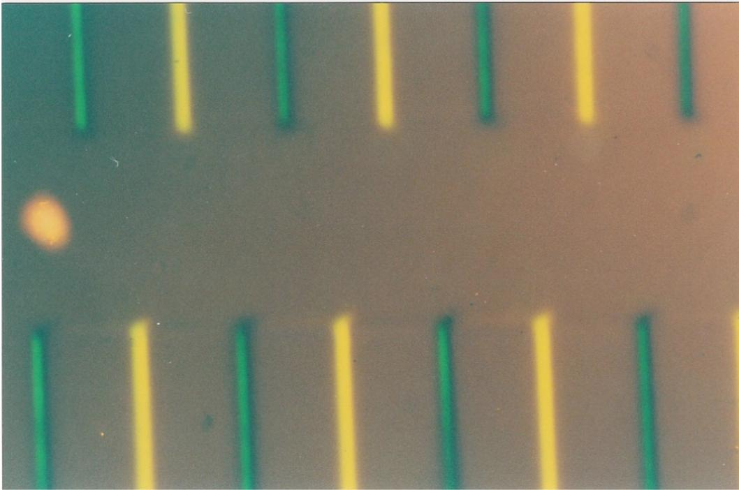
Fig. 5. Magnetooptic image of magnetic recording in a phone card.
