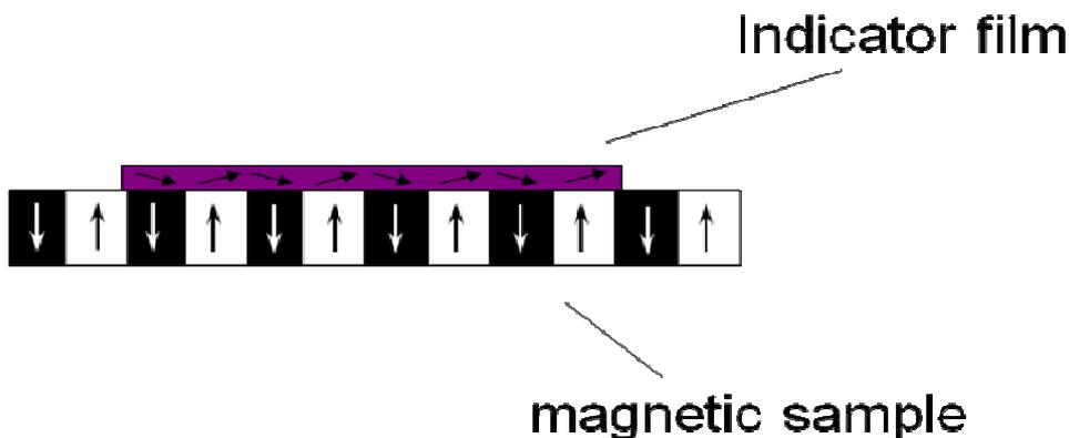
Fig. 3. Magnetization variation in in-plane YIG films placed on top of inhomogeneous magnetic sample.
