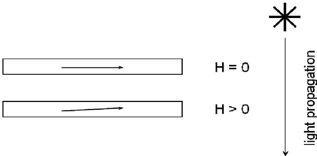
Fig. 2. Magnetization direction in in-plane YIG films
