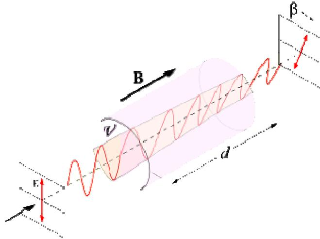
Fig. 1. Schematic representation of Faraday effect
